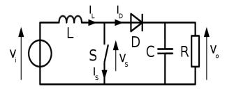
Figure 6: Boost Regulator Using Mosfet
