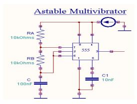
Figure 5: Astable Multivibrator Using 555 Timer
