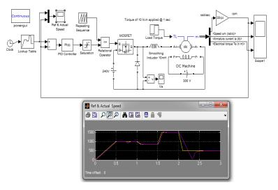
Chopper Fed DC Motor Drive -- Speed Control of DC motor
