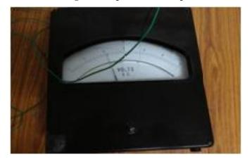
Figure 8: Output of Boost Regulator - The 3V DC Supply Fed to the Chopper Circuit is Converted Into 10.15V by the Boost Regulator
