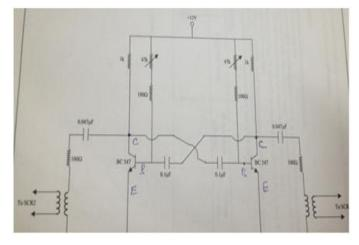
The circuit diagram for astable multivibrator is shown in Figure 3:
